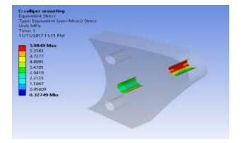
Fig -8: Caliper Mounting stress analysis
