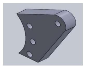
Fig -7: Caliper Mounting
