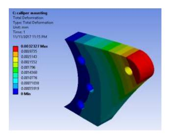
Fig -9 Caliper Mounting deformation analysis
