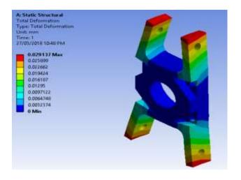
Fig -6: Rear upright Deformation analysis
