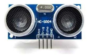
Fig -4: HC-SR 04 Ultrasonic Distance Sensor.
