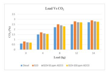
Fig-9: Variation of Carbon dioxide emissions with Load
