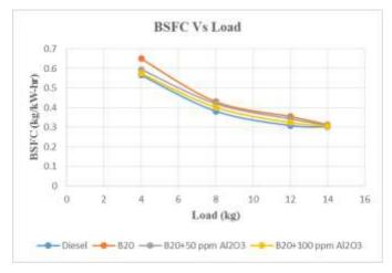
Fig-4: Variation of Specific fuel consumption with Load
