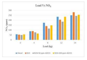
Fig-6: Variation of Nitrogen oxide emissions with Load
