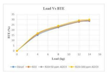
Fig-5 Variation of Brake thermal efficiency with Load
