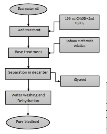
Fig-1: Flow chart of transesterification process
