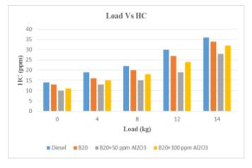
Fig-7: Variation of Hydrocarbon emissions with Load
