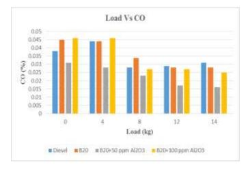
Fig-8: Variation of Carbon monoxide emissions with Load
