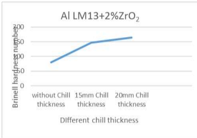
Chart 2.1.5: Effect of Cryogenic solidification on hardness
