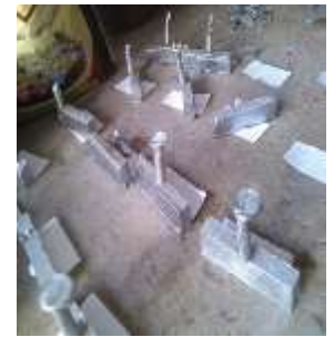
Figure 2.4: The solidified composite is separated by breaking the mould and placed according to weight percentage.
