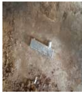
Figure 2.4: The solidified composite is separated by breaking the mould and placed according to weight percentage.
