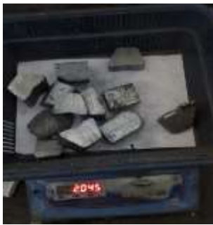
Figure 2.1: Aluminium alloy LM13 and Zirconium oxide weighing
