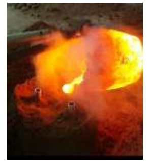
Figure 2.3: Passing of liquid nitrogen into the chill box and molten metal into the cavity
