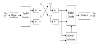
Fig-1: MIMO-OFDM system model
