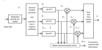
Fig -2: Block diagram of the PTS scheme with two transmit antennas
