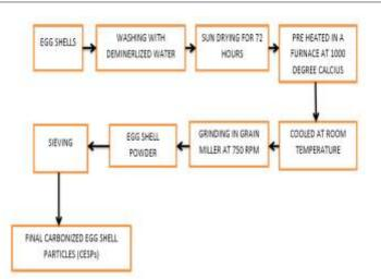
Fig.5. Process flow diagram
