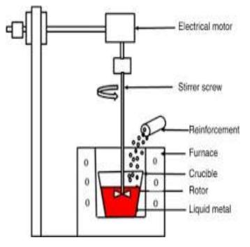
**Fig-4: Stir casting**
