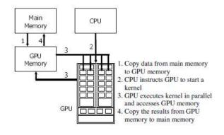
Fig -1: CUDA Threading Model
