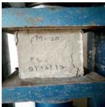
Fig -6: Compression Test in CTM
