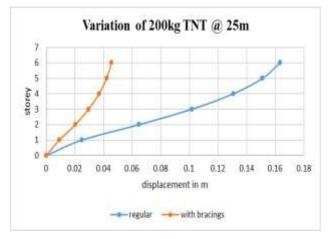
Fig 7: Storey displacement for 200 kg TNT at 25m
