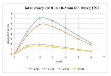
Fig 9: Storey drift for 100 kg TNT at 25m
