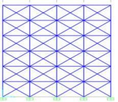
Fig 4: Building with bracings provided at outer periphery Section ISMB 200
