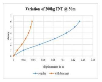
Fig 8: Storey displacement for 200kg TNT at 30m
