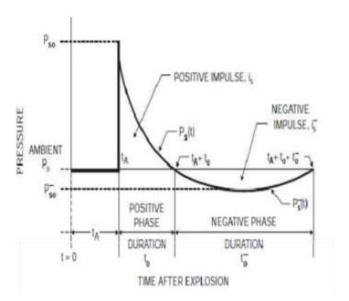
**Fig 1:** pressure variation with time after explosion
