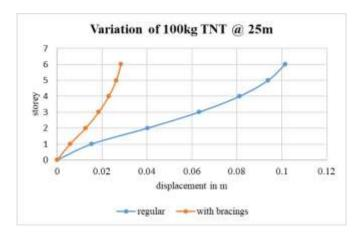
Fig 5: Storey displacement for 100 kg TNT at 25m
