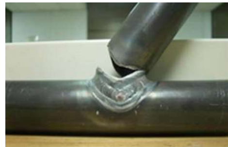
Fig -1: Failure of welded joint
