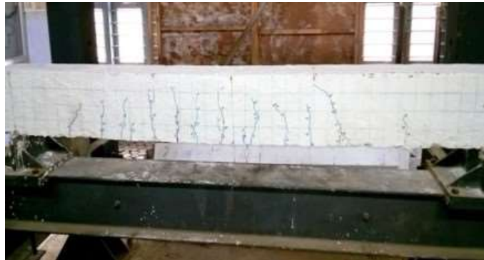
Fig-10 Crack pattern of Control Beam with Reduced Area reinforcement- CBRA
