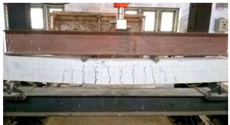
Fig -9 Crack pattern of Control Beam- CB
