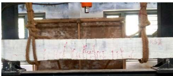
Fig -11 Crack pattern of Repaired Beam (RB @ 45)
