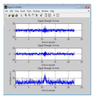
**Fig -1:** A typical simulated weather signal; time series and frequency spectra. (a) the in-phase component, I, (b) the quadrature component, Q,(c) the magnitude spectrum, |S(the square are root of the power spectrum on linear scale)
