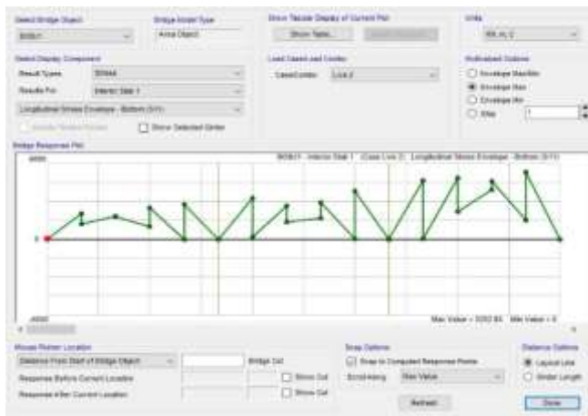
Fig 7 longitudinal stress at beams
