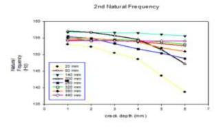
Fig -9: Variation of second natural frequency for various crack locations
