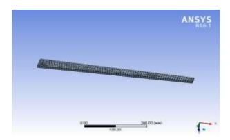
Fig -4: Meshing of healthy beam of ANSYS 16.1
