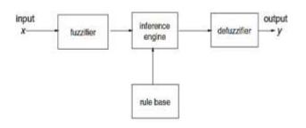
Fig- 2: Diagram of Fuzzy logic interference system
