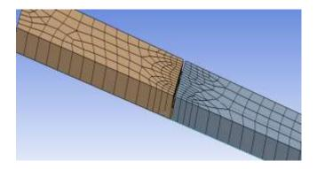
Fig -6: Meshing of the cracked portion
