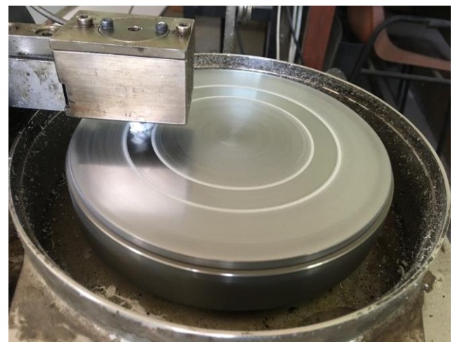
Fig-4: Wear test on pin-on-disc machine
