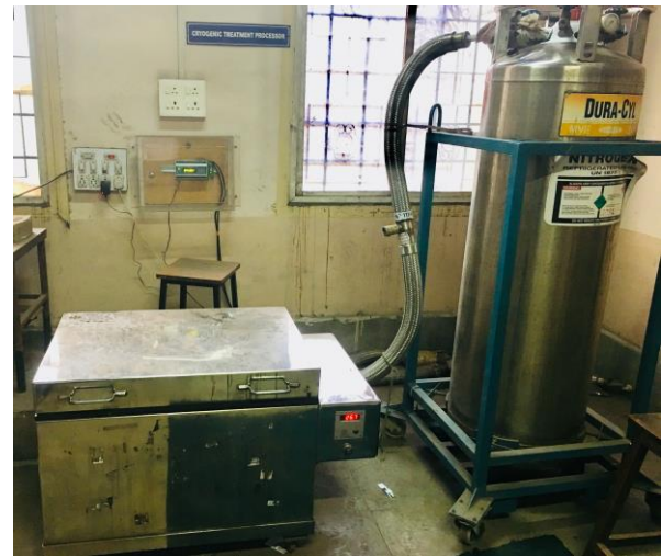
Fig-3: Complete setup for Cryogenic treatment
