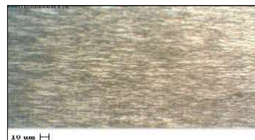
Fig-4.4 Microstructure of specimen at 1400rpm, 60mm/min.
