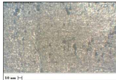
Fig-4.2 Microstructure of specimen at 900rpm, 40mm/min.
