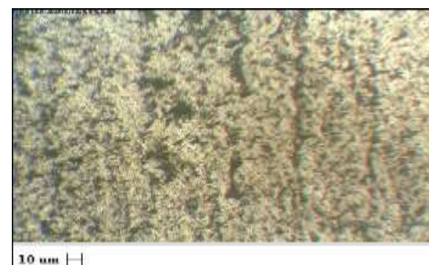
Fig-4.3 Microstructure of specimen at 1120rpm, 45mm/min.
