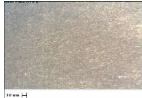
Fig-4.1 Microstructure of specimen at 700rpm, 30mm/min.
