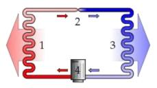
(Fig-9:Refrigeration system simple diagram)
