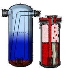
(Fig-5: Filter dryer)
