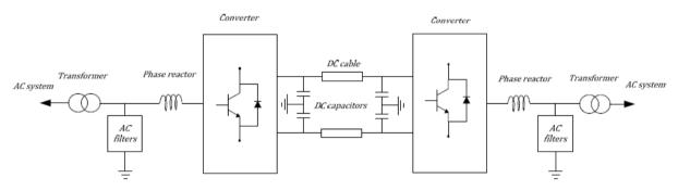
Fig-3 VSC-HVDC system configuration
