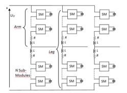
Fig-5: Schematic of a three-phase Modular Multilevel Converter
