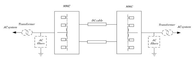
Fig-4: MMC-HVDC system configuration
