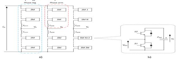
Fig-1 (a) Topology of three-phase MMC (b) Half-bridge sub-module
