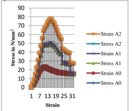
Comparison between Stress-Strain Curve of concrete having  $B_0(0,1)$ ,  $B_1(1,1)$  and  $B_2(2,1)$  deferent specimen (B Series)
