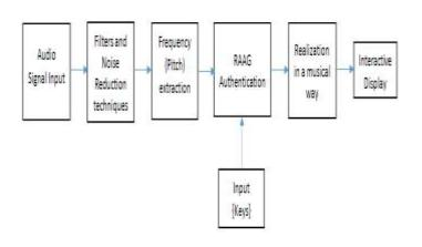
Fig -5: Block diagram / Flow of proposed system
