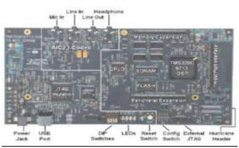
Fig -3: Board diagram of TMS320C6713 DSK
