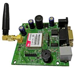
Fig -2.5: SIM800 GSM MODEM [2]
