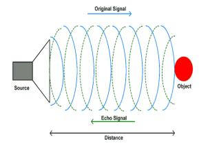
Fig -1.2: Ultrasonic Working Principle [2]
