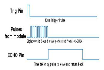
Fig -2.3: Ultrasonic Timing Diagram [2]
