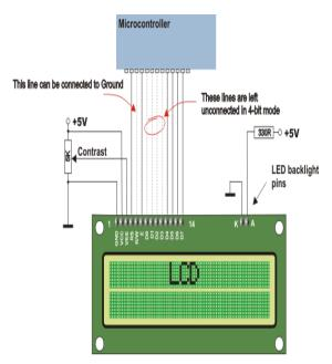
Fig -2.4: Connection of LCD Display with uC
