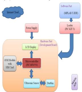
Fig -2.1: Block Diagram of Complete Project
