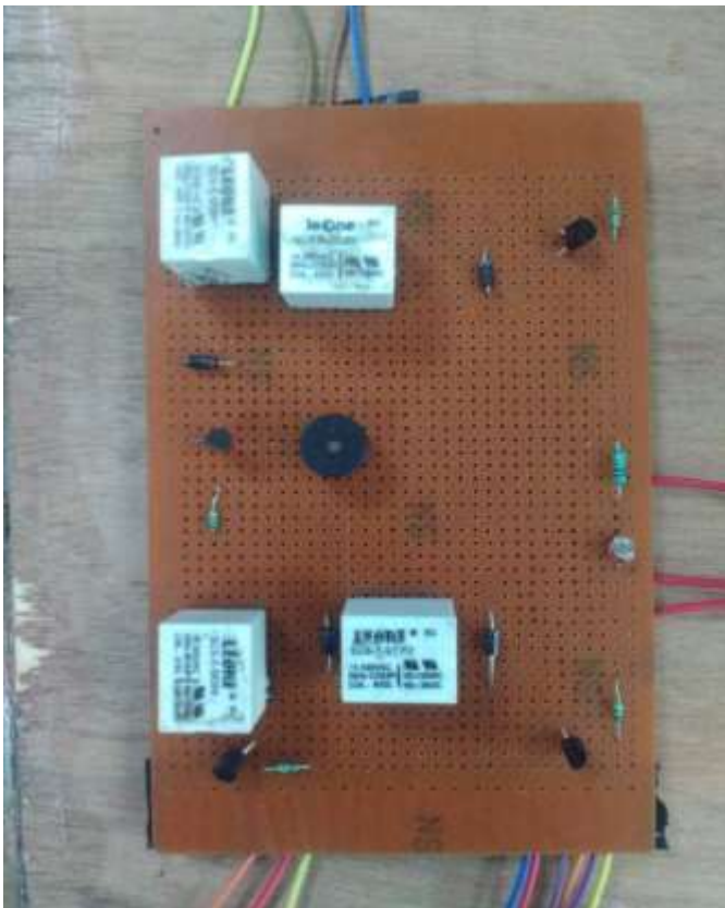
Fig. 3 Relay Circuit, Buzzer and Illumination Sensor
