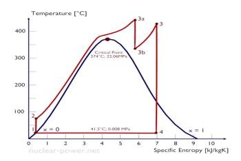
Fig. 1.2 Re heat Supercritical Rankine cycle
