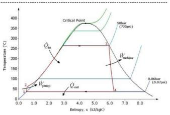
Fig1.1. Basic Rankine cycle (with various pressures)
