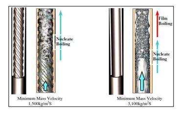
Fig. Rifled Tubes and Normal Tubes
