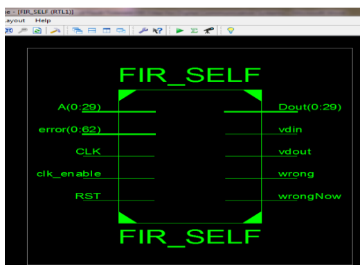
Figure 2: RTL view for Fault Tolerant FIR
