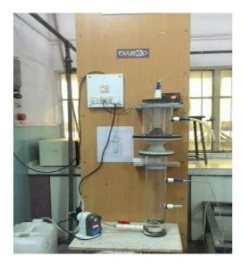
Fig. 1 Modified UASB reactor
