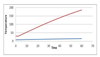
Graph-1: Max (red) and Min (blue) temperature variation in work roll for copper
