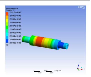
Fig-6 : Temperature on external surface at ( $\omega$ ) = 5 rad s<sup>-1</sup>
