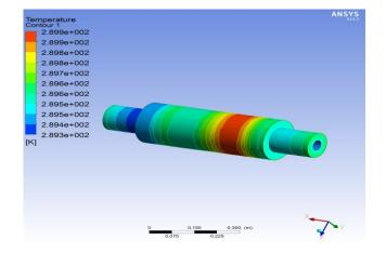
Fig-5 : Temperature on External surface at ( $\omega$ ) =15 rad s<sup>-1</sup>
