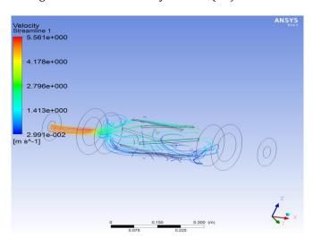
Fig-4: Fluid flow inside cylinder at ( $\omega$ ) = 5 rad s<sup>-1</sup>
