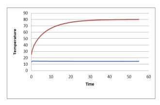
Graph-2: Max(red) and Min(blue) temperature variation in work roll for Aluminuium
