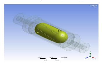
Fig-1: Internal cylinder with baffles construction
