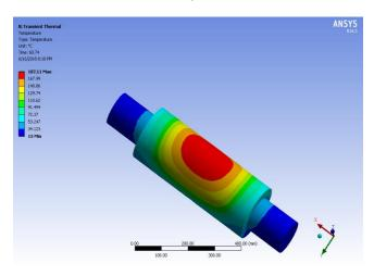
Fig-7: Temperature variation with Copper-Ethyl Glycol
