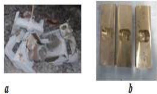
Fig.3.4 a. Replicast NAB Test plate in Knockout area after pouring. b. NAB three test plate for each process after machining.
