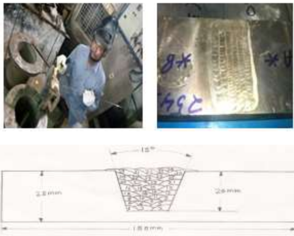
Fig.3.7 a. Ongoing GTAW-ACHF process of NAB P3 plate. b. NAB welded test plate P3. c. Welding sequence of GTAW-ACHF
