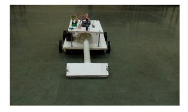
Fig -1: Front View of the Robot and the Vacuum Suction Pump
