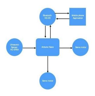
Fig -1: Block Diagram of the system
