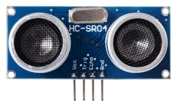
Fig -2: Ultrasonic Sensor (HC-SR04)
