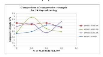
**Graph -3**: Compressive strength for 14 days cured compressed stabilized earth blocks in different chemical proportions
