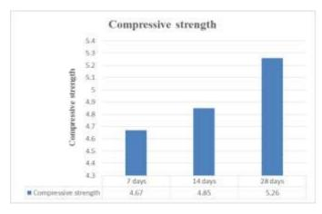
The result shows that the highest compressive strength of 5.260 N/mm<sup>2</sup> was obtained from sample at the curing age of 28 days.
