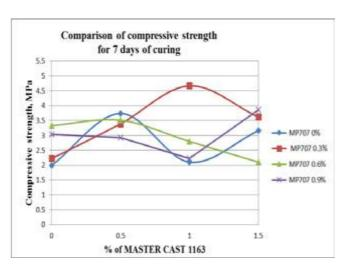
**Graph -2**: Compressive strength for 7 days cured compressed stabilized earth blocks in different chemical proportions
