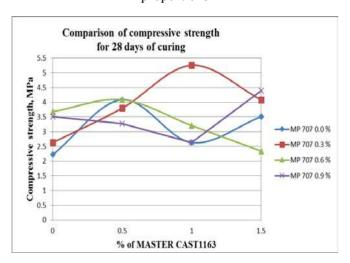
Graph -6: Compressive strength for 28 days cured compressed stabilized earth blocks in different chemical proportions.
