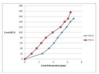
Fig-12: Load Vs Axial deformation graph of TFC-4
