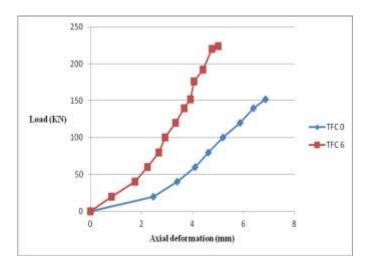
Fig-14: Load Vs Axial deformation graph of TFC-6
