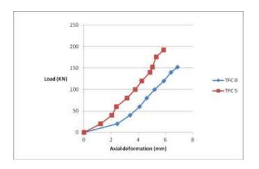
Fig.13 Load Vs Axial deformation graph of TFC-5
