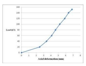
Fig-11: Load Vs Axial deformation graph of TFC-0
