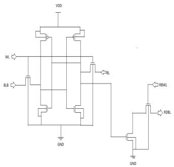
Fig 4.1 the circuit configuration of 8T SRAM Cell
