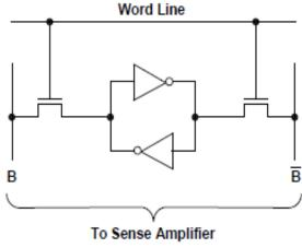
Fig 3.1 The SRAM Cell
