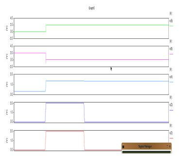
Fig 3.3 Write operation in the 7T SRAM Cell, storing "1" in the memory
