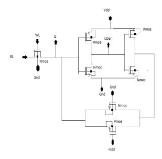
Fig 3.2 single ended input/output 7T SRAM cell
