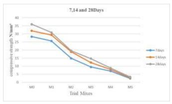
Fig 4.4 Compressive Strength Results for 7,14 and 28days
