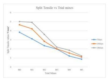
Fig 4.5 Split Tensile Strength Results for 7,14 and 28days of curing
