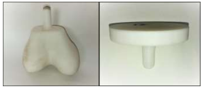
(A) (B) Fig.-2: 3D printed knee implant models on FDM, (A) Femoral implant, (B) Tibial implant.
