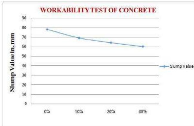
Graph 1: Workability testing of concrete Mix with CSA.
