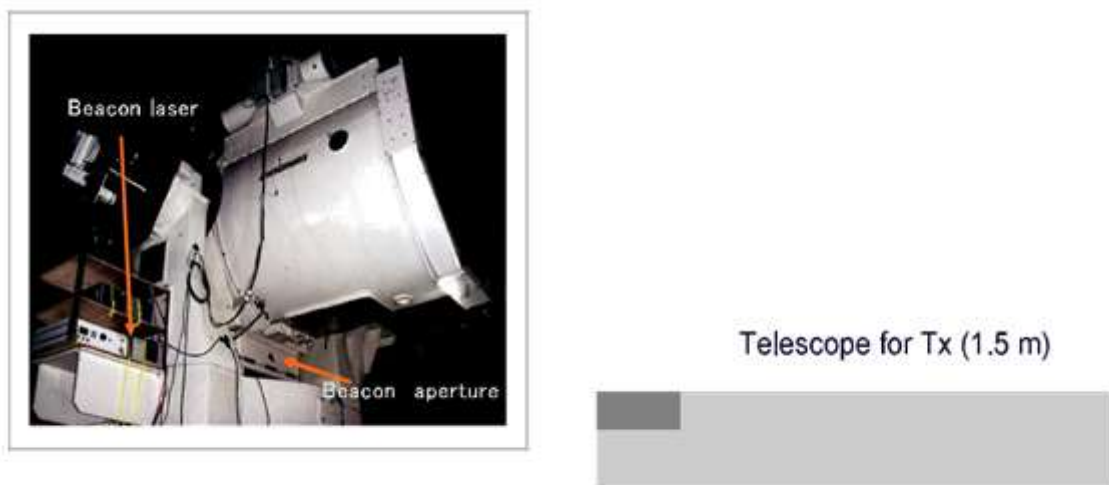
The 1.5-m telescope, the beacon laser source and the beacon aperture
