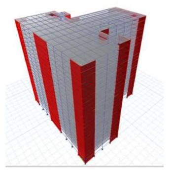
Fig-4: 3D view of T-shape structure with shear wall 4. MODEL DETAILS Bay in both direction: 8m No. of bays in both direction: 10 Storey height: 4m and 3.2m Stories: G+25 Concrete grade: M50-M25 www.irjet.net
