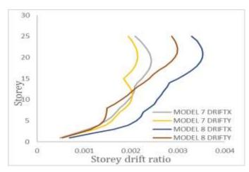
Chart -11: Storey drift ratio for M7 and M8
