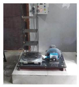
Fig -2: Setup without tuned liquid damper
