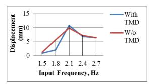
**Chart -3**: Variation of Displacement with excitation frequency ratio for TMD
