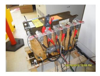
Figure 1.9: Snap picture of a 3-Phase100KVA Transformer under test.
