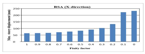
Fig. 11 : Maximum storey displacement predicted by RSA in X-direction
