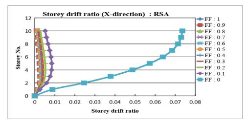
Fig. 8 : Variation of storey drift ratio for all the fixity factors predicted by RSA in X-direction
