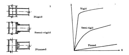
Fig. 1 : Types of beam-to-column connections
