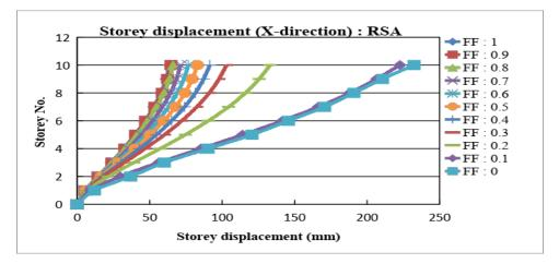
Fig. 6 : Variation of storey displacement for all the fixity factors predicted by RSA in X-direction
