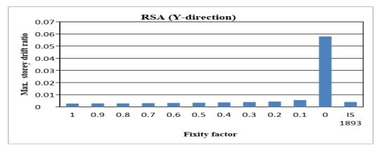
Fig. 14 : Maximum storey drift ratio predicted by RSA in Y-direction
