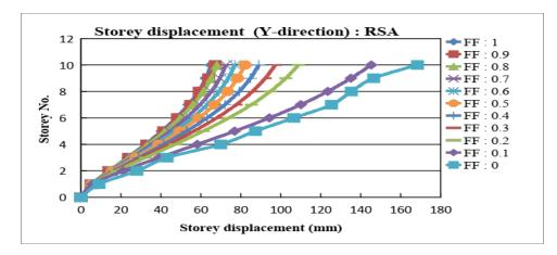
Fig. 7 : Variation of storey displacement for all the fixity factors predicted by RSA in Y-direction
