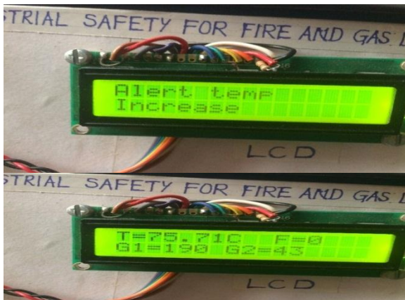
Figure 6 When the temperature exceeds the higher limits
