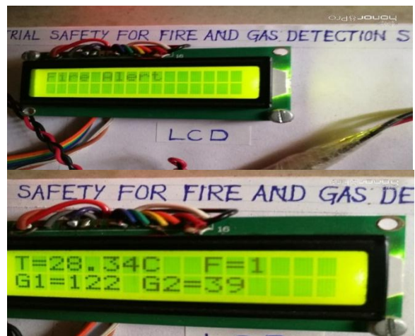
Figure 5 The fire is detected by the sensor.
