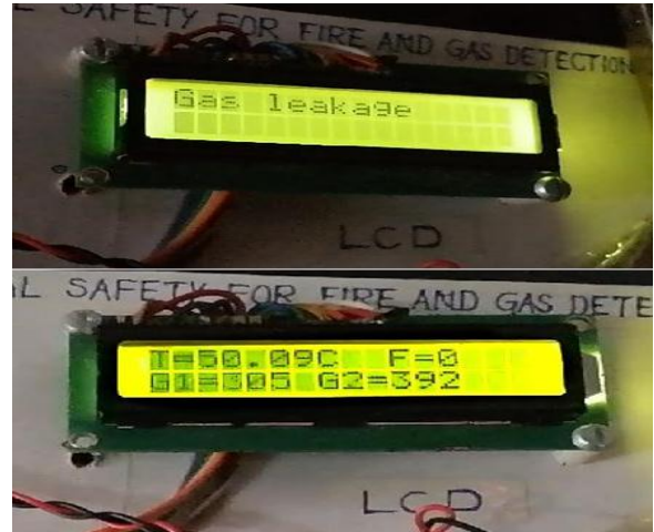
Figure 4. Gas leakage detected by gas sensor
