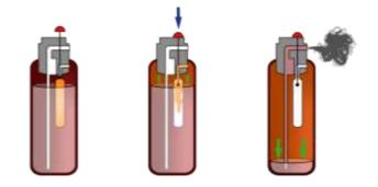
Fig -12: Working of a Sample Single-Stage Push-Button Extinguisher
