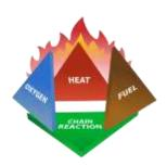
Fig -3: The Fire/Combustion Tetrahedron
