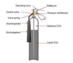
Fig -9: Carbon-dioxide Fire Extinguisher [10]
