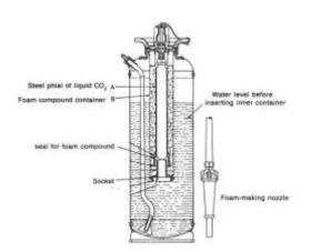
Fig -7: Foam Fire Extinguisher [10]
