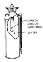
Fig -6: Water Fire Extinguisher [10]
