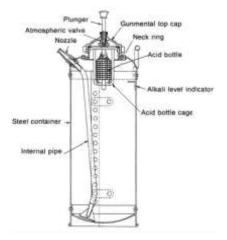
Fig -10: Wet Chemical Fire Extinguisher [10]
