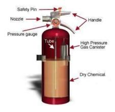
Fig -8: Dry Powder Fire Extinguisher [10]
