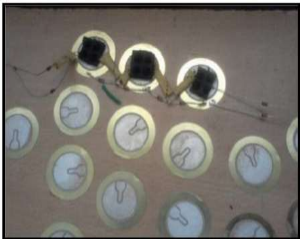
Fig -3: PZT in series connection
