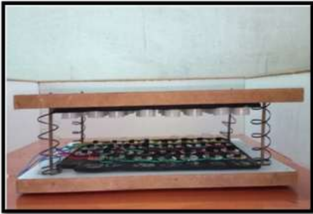
Fig -10: Final piezo material arrangement
