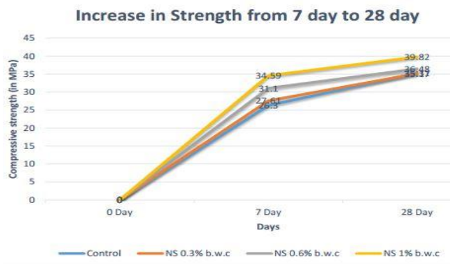
Fig. (e): Change in compressive strength of four specimen from 7 day to 28 day
