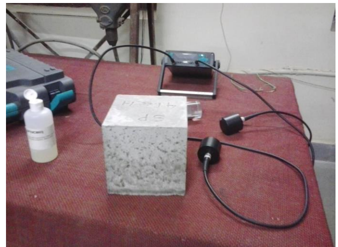
Fig. (b): UPV Test of concrete specimen Fig. (a) and (b) shows UPV Test performed in laboratory
