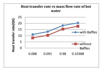
Chart -1: Heat transfer rate vs mass flow rate of hot water
