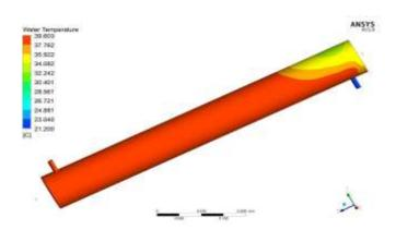
Figure 4: Temperature contour of water in shell
