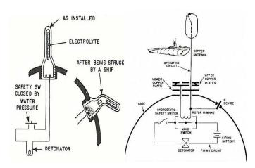
Fig. 2(a) & (b): Triggering by Hertz Horn and Antenna<sup>[4]</sup>
