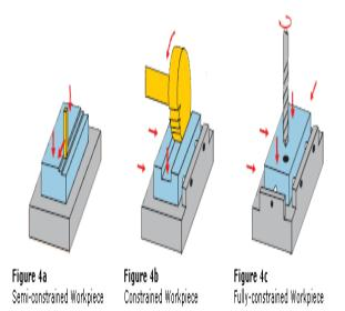
Fig.4: Work piece Placement
