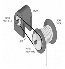
Fig.3: Power Transmission System
