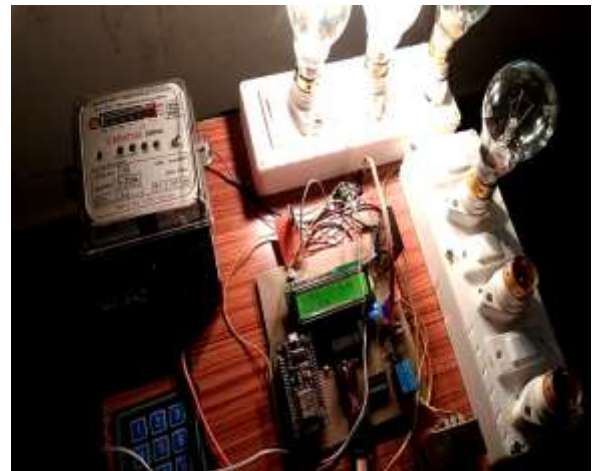
Fig. 7- System adjustment as per 200W loads at normal condition
