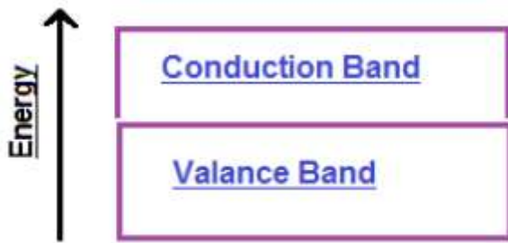
Fig-3:- Energy band diagram of Conductor
