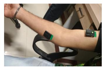
Fig -9: Sensors placed on both the concerned muscles using double-sided adhesive tapes.
