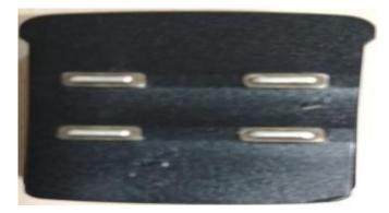
Fig -7: 4- channel Ag/AgCl electrodes used on the sensor
